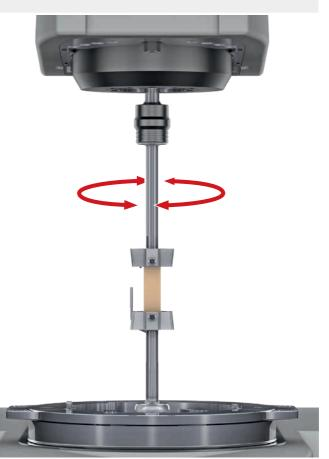
In this mode the linear drive is brought into a fixed position, while the rotational drive is used to control shear strain or shear stress. In combination with available fixtures such as solid circular and rectangular fixtures (SCF, SRF) and plate-plate or cone-plate geometries, this option opens up the possibility to perform dynamic mechanical analysis in torsion and also rheological measurements.
