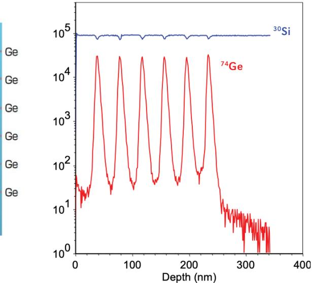
A depth profile of a multi delta layer (MDL) sample of Ge in Si was acquired using a 30 keV  $\text{Bi}^+$  primary ion beam (50  $\mu\text{m}$  square raster) and a 1 keV  $\text{Cs}^+$  sputter ion beam (200  $\mu\text{m}$  square raster). The Ge delta layers are 0.4 nm thick.
