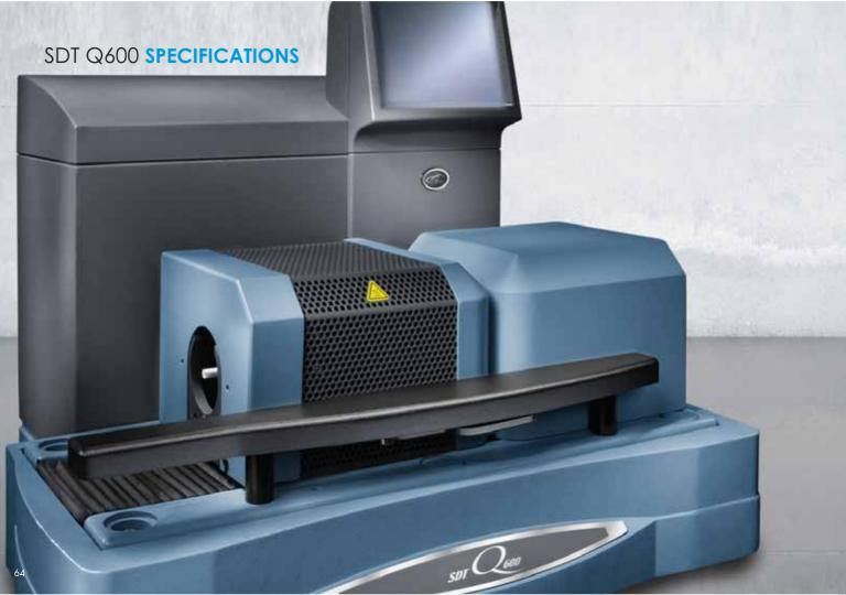
The Q600 provides simultaneous measurement of weight change (TGA) and true differential heat flow (DSC) on the same sample from ambient to 1,500 °C. It features a field-proven horizontal dual beam design with automatic beam growth compensation, and the ability to analyze two TGA samples simultaneously. DSC heat flow data is dynamically normalized using the instantaneous sample weight at any given temperature.
