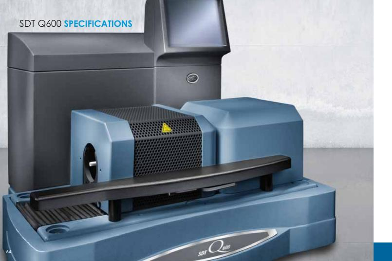
The Q600 provides simultaneous measurement of weight change (TGA) and true differential heat flow (DSC) on the same sample from ambient to 1,500 °C. It features a field-proven horizontal dual beam design with automatic beam growth compensation, and the ability to analyze two TGA samples simultaneously. DSC heat flow data is dynamically normalized using the instantaneous sample weight at any given temperature.
