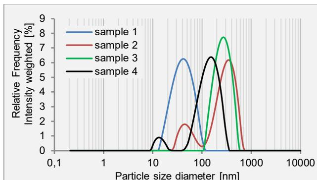
Figure 3: Intensity weighted particle size distribution of four CBD emulsion samples. Mean values of three consecutive measurements are displayed.
