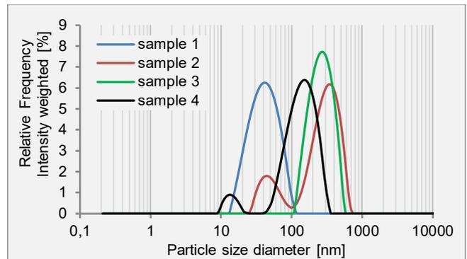
Figure 3: Intensity weighted particle size distribution of four CBD emulsion samples. Mean values of three consecutive measurements are displayed.
