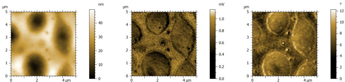
Figure 2. Height (left), amplitude (middle) and phase (right) images acquired by CR Amplitude Imaging
