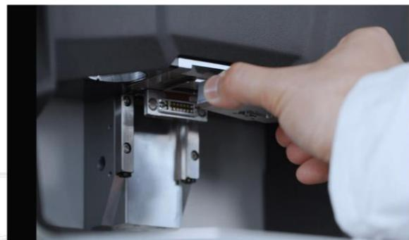
Inserting the actuator body with the cantilever
