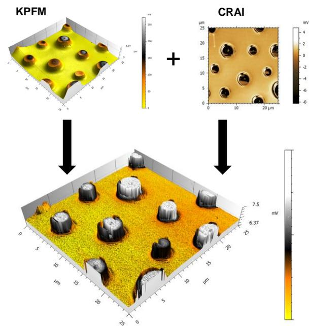
Superposition of 3D CRAI amplitude and contact potential difference (CPD)
