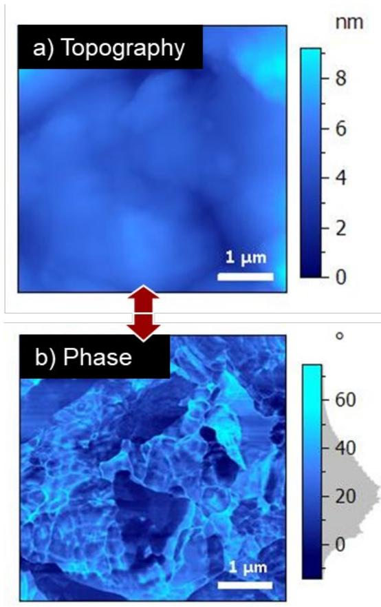
Figure 4: a) 5x5 µm AFM topography (forward trace) image of the glove surface showing no particular differentiation in materials. b) Phase (forward trace) image of the same region showing regions of different materials, possibly the filler or pigment added to the rubber.
