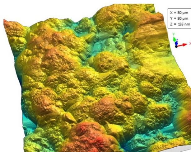
Figure 3: An 80x80 µm 3-D topography (forward trace) AFM image of the nitrile glove surface.
