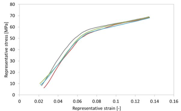
Figure 7 - Comparison of indentation stress-strain curves on a polymer (NHT<sup>3</sup> with  $R = 20 \mu\text{m}$  spherical indenter, measurements in Sinus mode).
