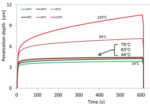
Figure 10 – Creep data (penetration depth increase during 10-minutes hold at constant force). Note large increase at 94°C and 110°C.
