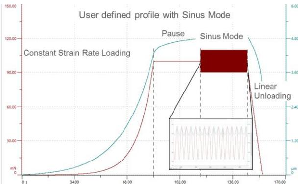
Figure 2 – Typical loading profile for Sinus mode measurement on polymers.
