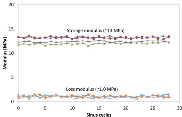
Figure 3 – Typical loading profile for Sinus mode measurement on polymers (PVB sample).
