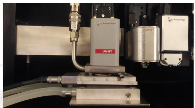
Figure 8 – The UNHT<sup>3</sup> with water cooling block and the  $200^\circ\text{C}$  heating module.
