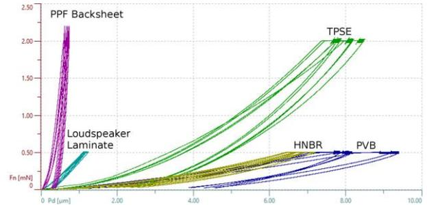
Figure 4 – Comparison of Sinus mode tests on five polymeric sheets: TPSE Encapsulant, Loudspeaker laminate, PPF Backsheet, PVB and HNBR.
