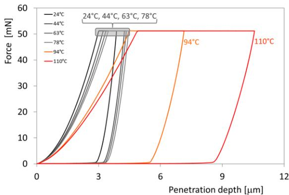
Figure 9 – Nanoindentation of PMMA at different temperatures. Note large increase in penetration depth as well as increase of creep at 94°C and 110°C.
