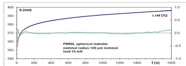
Figure 5 – UNHT<sup>3</sup> Creep measurement with fit and residuals ( $\Delta rel$ ) on polyacrylamide (PMMA). Maximum load 10 mN, duration of creep 1800 s, depth increase during hold ~30 nm.
