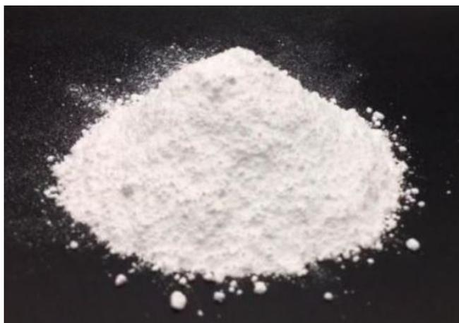
Figure 1: PTFE powder. Notice the inherent clumping (due to its fluorine molecule interactions), even though it is hydrophobic in nature.
