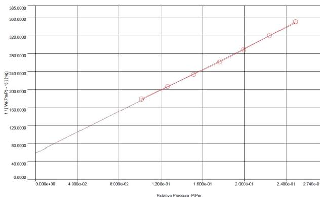
Figure 3: BET surface area of PTFE powder :  $2.59 \text{ m}^2/\text{g}$ .
