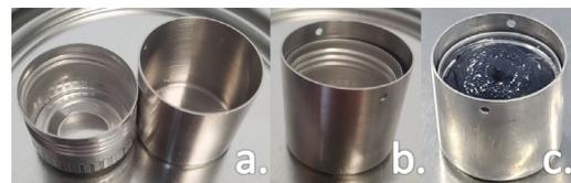
Figure 1: Disposable aluminum cup next to (a.) and inside of (b.) the small sample cell. The prepared sample cell is shown in (c.).
