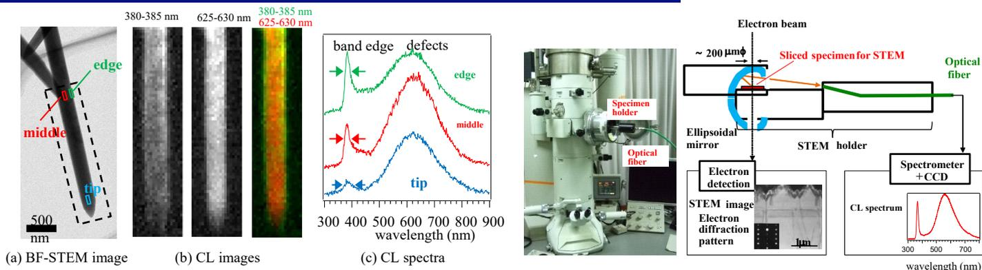
Figure 1-1. (a) BF-STEM, (b) CL images at various wavelengths, and (c) CL spectra of ZnO NW
