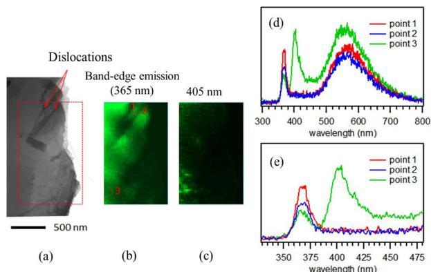
Fig. 2-2. (a) STEM, (b) CL image at 365 nm, and (c) CL image at 405 nm in the scanning area of  $1 \mu\text{m} \times 2 \mu\text{m}$ , and the CL spectra at points 1-3 from (d) 300 nm to 800 nm, and (e) from 325 nm to 476 nm of a GaN crystal.
