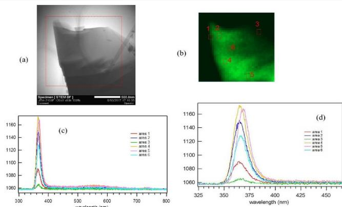
Fig.2-1. (a) STEM and (b) CL intensity image (365-nm peak) in a scanning area of  $1 \mu\text{m} \times 2 \mu\text{m}$ , and CL spectra at points 1-6 (c) from 300 to 800 nm and (d) from 325 to 465 nm of a piece of GaN crystal flake with a thickness of less than 100 nm, measured by an acceleration voltage of 120 keV.
