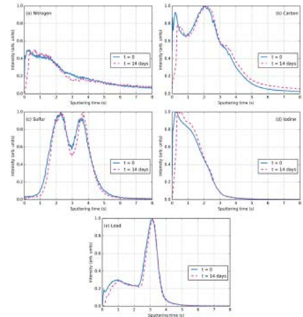
Direct comparison of the elemental distribution at first exposure to air (continuous blue curve) and after 14 days of exposure to air (hatched pink curve) for (a) nitrogen, (b) carbon, (c) sulfur, (d) iodine and (e) lead.
