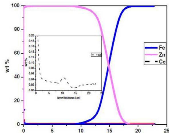
Pulsed RF GDOES depth profile (insert: the distribution in the layer)
