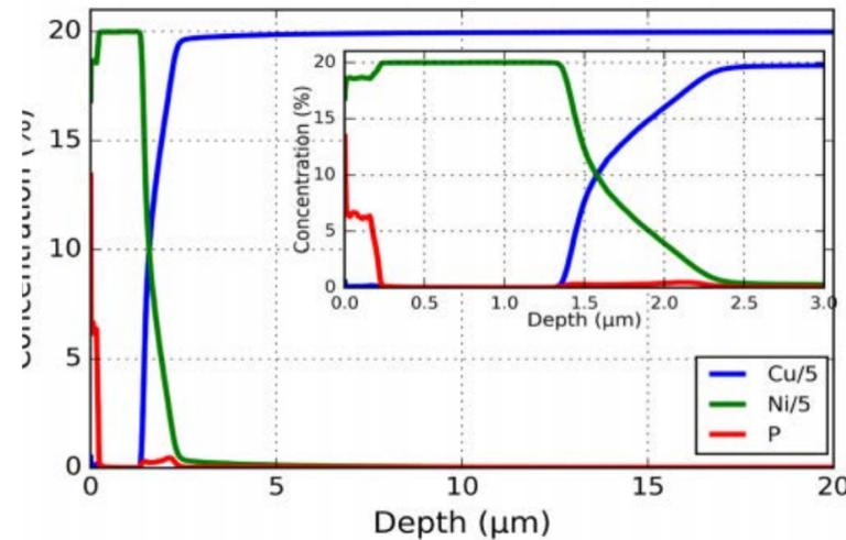
Quantified elemental depth profile for the sample shown. By establishing a set of calibration curves, it has been possible to convert the relative GDOES analysis presented in a quantitative result.
