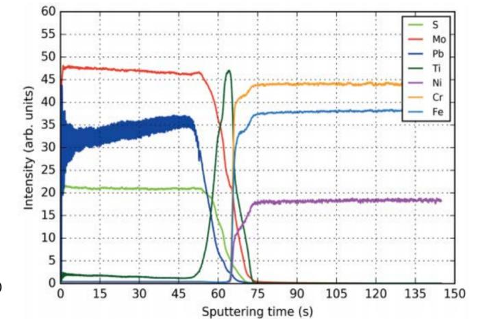
Full depth profile of MoS<sub>2</sub>/Pb coating obtained with the GD Profiler 2
