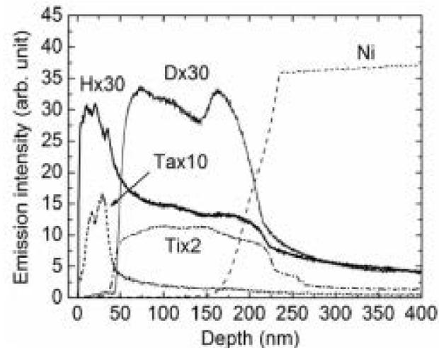
Depth profiles of H, D, Ta, Ti and Ni in the Tz(H)Ti(D)/Ni layered structure
