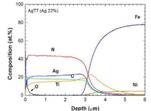
GD depth profile of a coating deposited by magnetron sputtering
