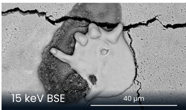
Figure 4: BSE images of Tantalum hand on a barium/carbon/oxygen oval on a cracked iron/tantalum/silicon substrate taken with different accelerating voltages. From Covalent Metrology's Covalent Academy webinar #18.
