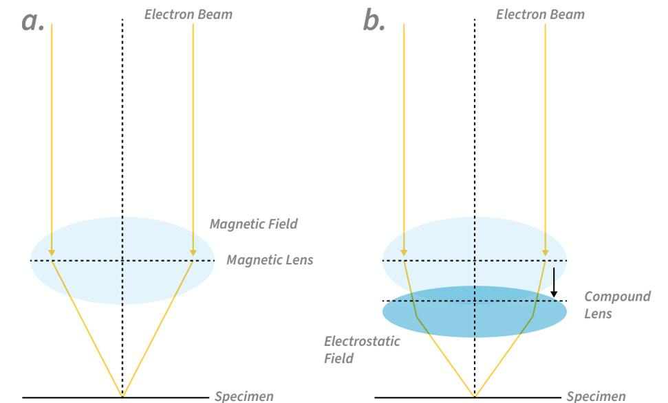
*Difference of the electron probe on the specimen for the magnetic objective lens and for the electrostatic/electromagnetic field superposed objective lens.*
