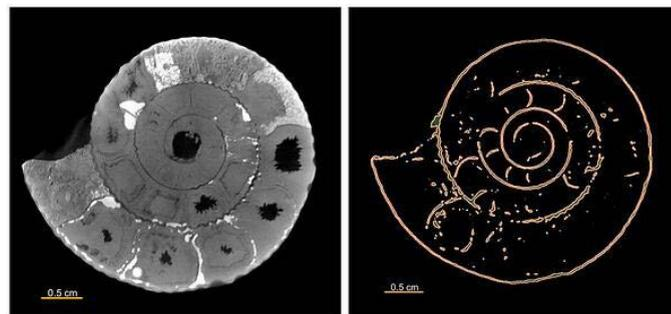
CT scan of an ammonite fossil (Perisphinctes). CT cross-section (left) and extracted surface mesh (right).
