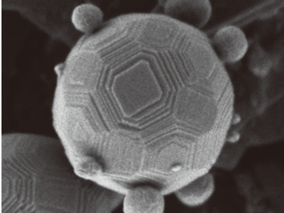
Specimen: Aluminium Oxide particles, Accelerating voltage: 0.5 kV, Observation mode: BD, Detector: UHD
